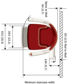
Minimum staircase width driven by footrest 654mm (25.7) Arm dimension 652mm (25.6)
