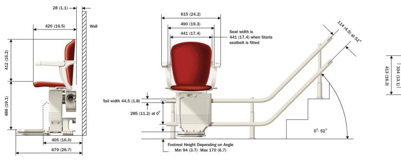
All product dimensions are accurate, however, you should add approximately 30mm on dimensions that require clearance for the user, such as the minimum swivel width dimension.
