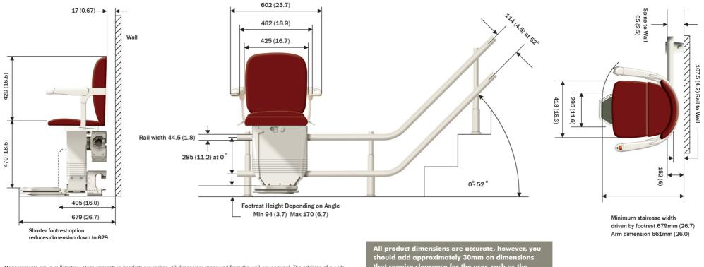
Measurements are in millimetres. Measurements in brackets are inches. All dimensions measured from the wall are nominal. The addition of a wide stringer or similar obstruction may affect the dimensions taken from this point. The colour representation of the chair shown here is for illustrative purposes only. Weight limit note: Upto 135kg - approx 21 stone / 297 lbs. Powered hinge is limited to 120kg - approx 19 stone / 265 lbs.
